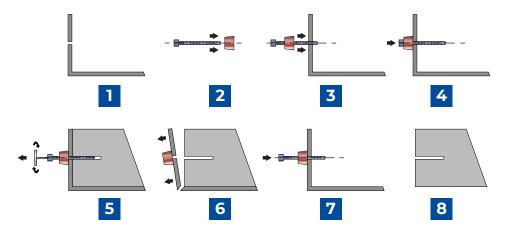
Seal the remaining holes in concrete with Innogain MB cover caps if required.
