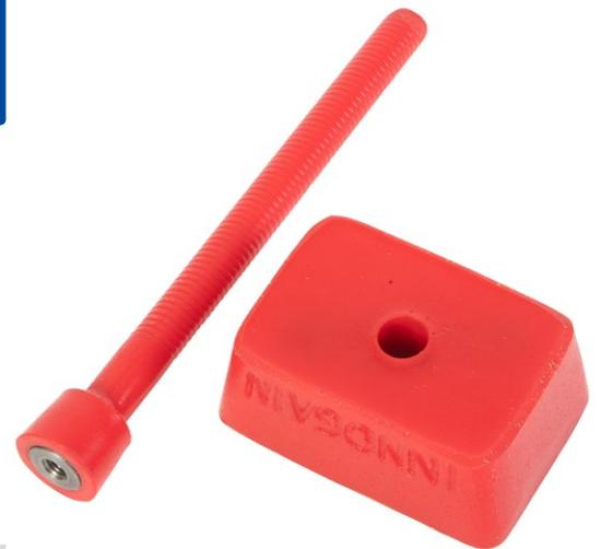
**1** To use the InnoGain 3D system on the formwork there has to be a hole in it of  $\varnothing 14\text{mm}$  with no sharp edges. This is very important because the InnoGain MGM is tapered  $\varnothing 14-14,5$  so the MGM has to be pressed a little bit through the hole of the formwork.
